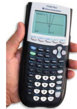
Figure 1.9 A typical graphing calculator by Texas Instruments, displaying a graph of a function f(x) = 2x^2 - 3 .
